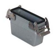
Hood, V-TYPE series, with 2 levers, Pg21 top cable entry without adapter, size "77.27", high construction
