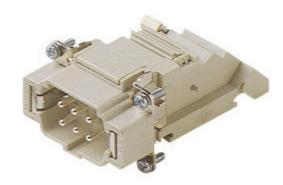
Male insert, CTSE series, spring terminal connection, 6 poles + PE, 16 A 500 V 6 kV 3, size "44.27", with incorporated terminal block, left side mounting
