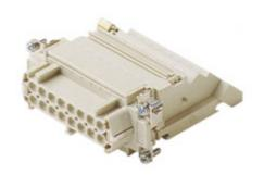
Female insert, CT series, screw terminal connection, 16 poles + PE, 16 A 230/400 V 4 kV 2, size "77.27", with incorporated terminal block, left side mounting
