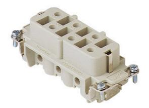
Female insert, CP series, screw terminal connection, 6 poles + PE, 35 A 400/690 V 6 kV 3, size "77.27", without plate
