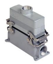
Complete connector, CNZ series, composed of 2 screw terminal connection inserts with 24 poles + PE, and surface mounting housing with 2 levers and hood with top cable entry
