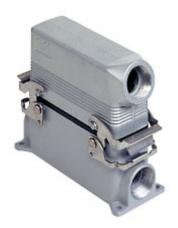
Complete connector, CNZ series, composed of 2 screw terminal connection inserts with 24 poles + PE, and surface mounting housing with 2 levers and hood with side cable entry
