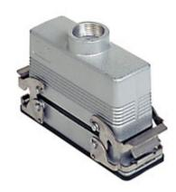
Complete connector, CNZ series, composed of 2 screw terminal connection inserts with 24 poles + PE, and bulkhead mounting housing with 2 levers and hood with top cable entry
