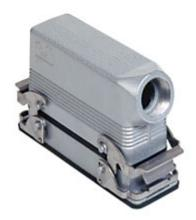
Complete connector, CNZ series, composed of 2 screw terminal connection inserts with 24 poles + PE, and bulkhead mounting housing with 2 levers and hood with side cable entry
