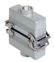
Complete connector, CNZ series, composed of 2 screw terminal connection inserts with 16 poles + PE, and hoods with top cable entry and closing with 2 levers
