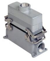
Complete connector, CNZ series, composed of 2 screw terminal connection inserts with 16 poles + PE, and surface mounting housing with 2 levers and hood with top cable entry
