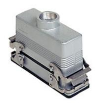
Complete connector, CNZ series, composed of 2 screw terminal connection inserts with 16 poles + PE, and bulkhead mounting housing with 2 levers and hood with top cable entry
