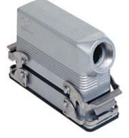
Complete connector, CNZ series, composed of 2 screw terminal connection inserts with 16 poles + PE, and bulkhead mounting housing with 2 levers and hood with side cable entry
