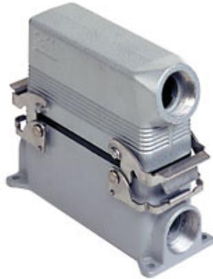
Complete connector, CNZ series, composed of 2 screw terminal connection inserts with 10 poles + PE, and surface mounting housing with 2 levers and hood with side cable entry
