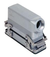
Complete connector, CNZ series, composed of 2 screw terminal connection inserts with 10 poles + PE, and bulkhead mounting housing with 2 levers and hood with side cable entry
