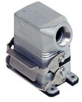
Complete connector, CNZ series, composed of 2 screw terminal connection inserts with 24 poles + PE, and bulkhead mounting housing with 1 lever and hood with side cable entry
