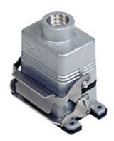
Complete connector, CNZ series, composed of 2 screw terminal connection inserts with 16 poles + PE, and bulkhead mounting housing with 1 lever and hood with top cable entry
