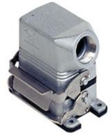
Complete connector, CNZ series, composed of 2 screw terminal connection inserts with 10 poles + PE, and bulkhead mounting housing with 1 lever and hood with side cable entry
