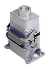
Complete connector, CNZ series, composed of 2 screw terminal connection inserts with 6 poles + PE, and surface mounting housing with 1 lever and hood with top cable entry
