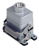
Complete connector, CNZ series, composed of 2 screw terminal connection inserts with 6 poles + PE, and bulkhead mounting housing with 1 lever and hood with top cable entry
