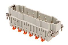
Male insert, CMSH series, SQUICH® spring terminal connection without tools, 10+2 poles + PE (25-48), 16 A 830 V 8 kV 3 / 16 A 500 V 6 kV 3, size "104.62"
