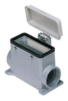
Surface mounting housing, 830V series, with 4 pegs, Pg21 cable entry, size "77.27", with plastic cover
