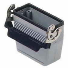
Hood, 830V series, with 1 lever, Pg21 top cable entry without adapter, size "104.27", high construction
