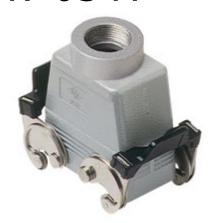
Hood, 830V series, with 2 levers, Pg21 top cable entry, size "57.27", high construction, without gasket
