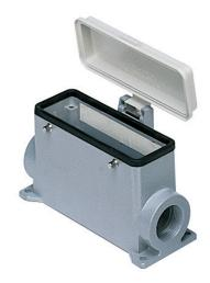
Surface mounting housing, 830V series, with 4 pegs, Pg29 x 2 cable entry, size "104.27", high construction, with plastic cover
