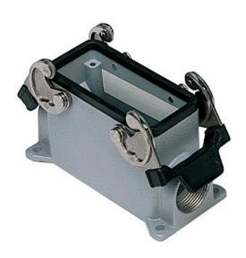
Surface mounting housing, 830V series, with 2 levers, Pg21 x 2 cable entry, size "77.27", high construction
