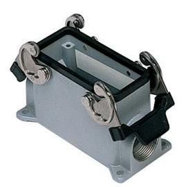
Surface mounting housing, 830V series, with 2 levers, Pg29 cable entry, size "57.27", high construction
