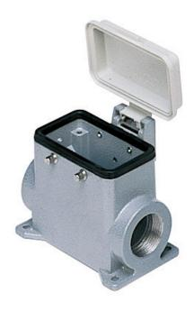
Surface mounting housing, 830V series, with 4 pegs, Pg29 cable entry, size "57.27", high construction, with plastic cover
