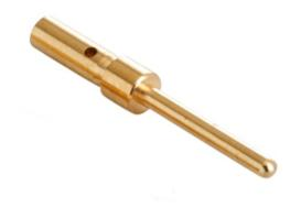
Male crimp contact, CI series, 5 A, turned gold plated, wire cross section 0,08 - 0,13 mm<sup>2</sup>, AWG 28 - 26, for D-SUB connectors
