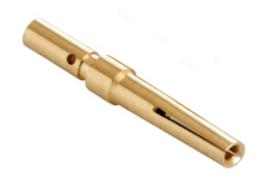
Female crimp contact, CI series, 5 A, turned gold plated, wire cross section 0.32 - 0.82 mm<sup>2</sup>, AWG 22 - 18
