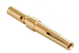
Female crimp contact, CI series, 5 A, turned gold plated, wire cross section 0,2 - 0,52 mm², AWG 24 - 20, for D-SUB connectors
