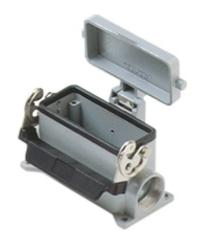
Surface mounting housing, C-TYPE series, with 1 lever, Pg21 x 2 cable entry, size "77.27", with metal cover
