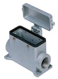
Surface mounting housing, C-TYPE series, with 4 pegs, Pg21 cable entry, size "77.27", with metal cover
