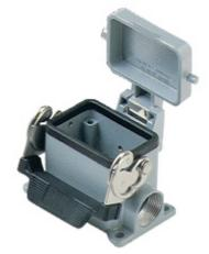
Surface mounting housing, C-TYPE series, with 1 lever, Pg16 cable entry, size "44.27", with metal cover
