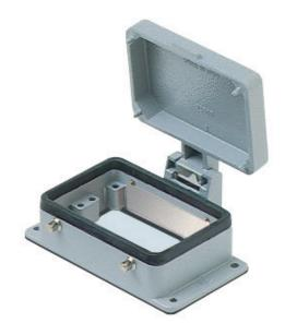
Bulkhead mounting housing, C-TYPE series, with 4 pegs, size "66.40", with metal cover
