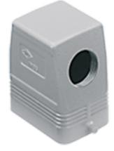
Hood, C-TYPE series, with 2 pegs, Pg29 side cable entry without adapter, size "44.27", high construction
