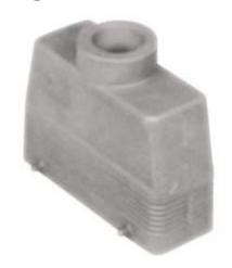
Hood, EMC series, with 2 pegs, Pg21 top cable entry, size "104.27", high construction
