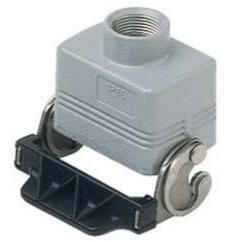
Hood, C-TYPE series, with 1 lever, Pg21 top cable entry, size "44.27", high construction, without gasket
