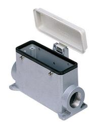
Surface mounting housing, C-TYPE series, with 4 pegs, Pg21 cable entry, size "104.27", high construction, with plastic cover
