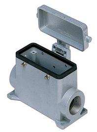
Surface mounting housing, C-TYPE series, with 4 pegs, Pg21 cable entry, size "77.27", high construction, with metal cover
