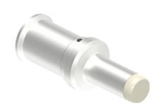
Male crimp contact, C30 series, 300 A, turned silver plated, wire cross section 95 mm<sup>2</sup>, AWG 3/0, finger-proof version
