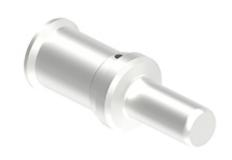
Male crimp contact, C30 series, 300 A, turned silver plated, wire cross section 95 mm<sup>2</sup>, AWG 3/0
