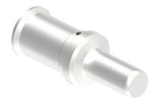
Male crimp contact, C30 series, 300 A, turned silver plated, wire cross section 70 mm<sup>2</sup>, AWG 2/0
