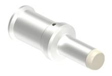
Male crimp contact, C30 series, 300 A, turned silver plated, wire cross section 50 mm<sup>2</sup>, AWG 1, finger-proof version
