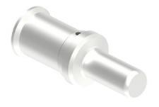
Male crimp contact, C30 series, 300 A, turned silver plated, wire cross section 50 mm<sup>2</sup>, AWG 1
