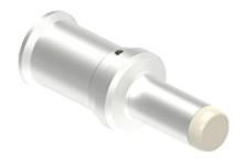
Male crimp contact, C30 series, 300 A, turned silver plated, wire cross section 25 mm<sup>2</sup>, AWG 4, finger-proof version
