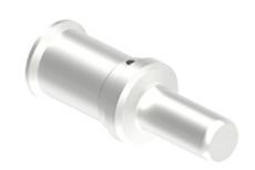
Male crimp contact, C30 series, 300 A, turned silver plated, wire cross section 120 mm<sup>2</sup>, AWG 4/0
