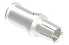
Female crimp contact, C30 series, 300 A, turned silver plated, wire cross section 70  $mm^2$ , AWG 2/0
