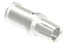
Female crimp contact, C30 series, 300 A, turned silver plated, wire cross section 35  $mm^2$ , AWG 2
