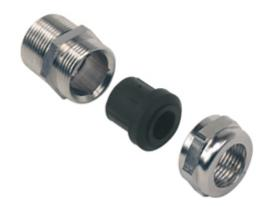
Complete cable gland, M25, for diameter 11,5-18 mm, 15 mm threading length
