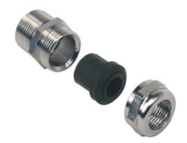
Complete cable gland, Pg11, for diameter 6-10 mm, 15 mm threading length
